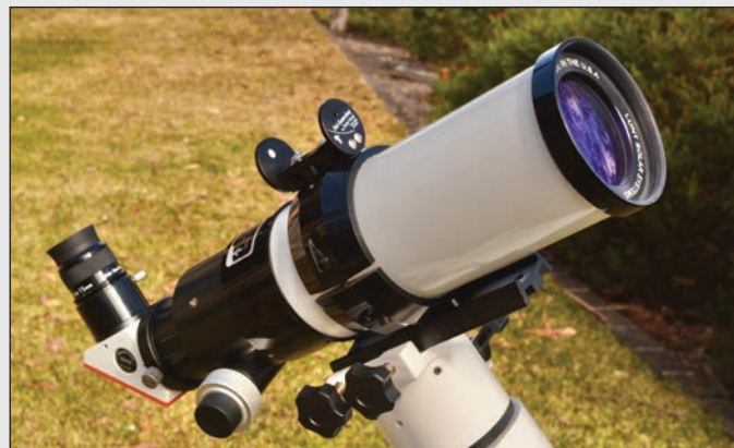
A 60 mm dedicated Hydrogen Alpha telescope
