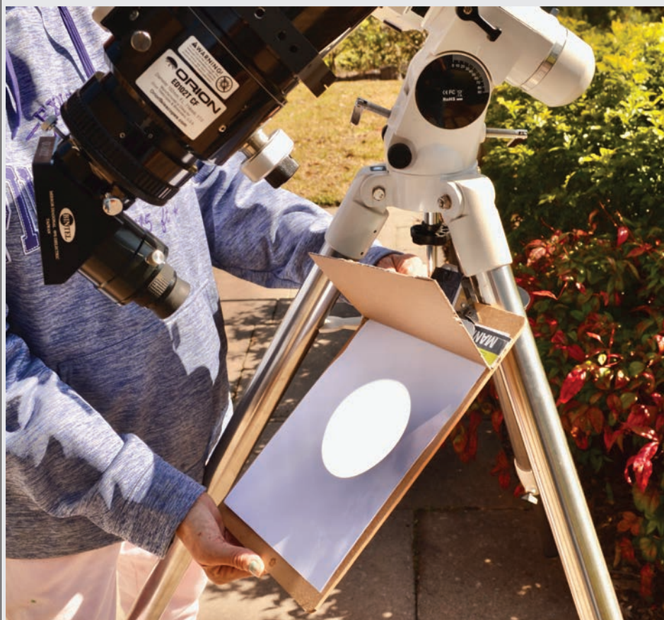
Projecting the Sun's image with a refracting telescope.
