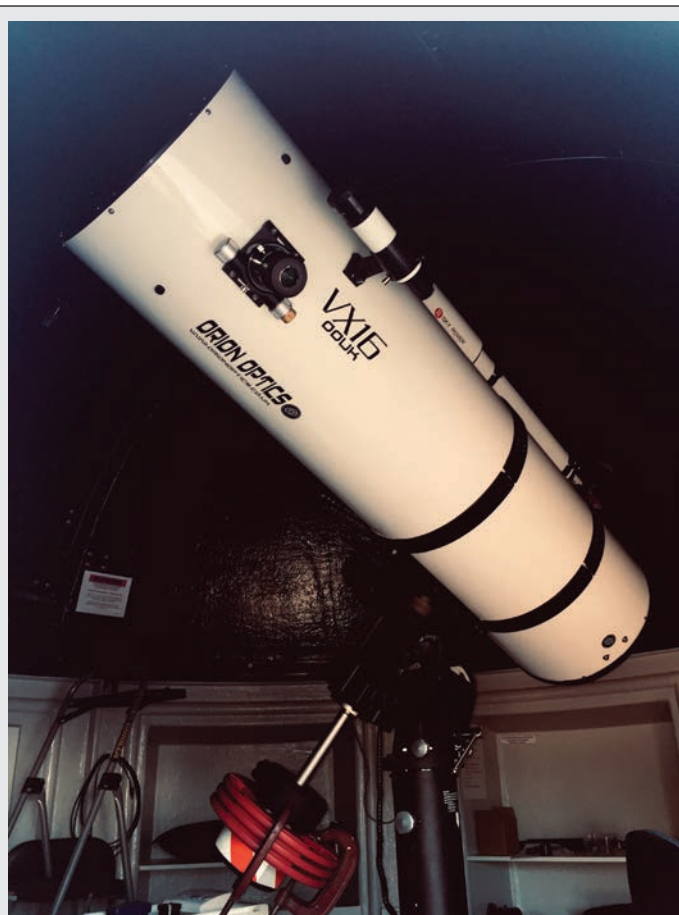
MSATT-2, Orion Optics 400 mm f4 Newtonian
