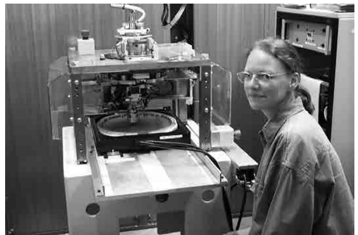
Figure 3. The 6dF robot positioning optical fibres under the watchful eye of UK Schmidt Telescope observer Kristin Fiegert. The robot positions the fibres so that they will be in alignment with RAVE target stars when loaded into the telescope (Courtesy Jonathan Pogson, Anglo-Australian Observatory).
