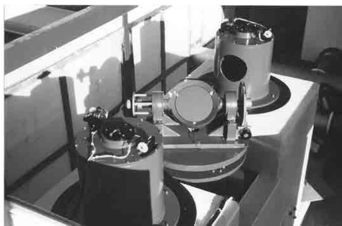
A siderostat station, showing the 20cm mirror in its alt-az mounting (the siderostat), which feeds starlight into one of the north or south periscopes mounted on either side of it.
